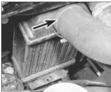
22.3 Intercooler upper air hose attachment (arrowed)
