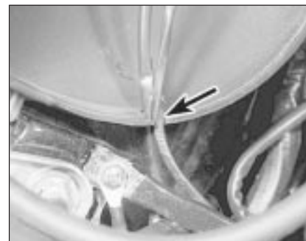
16.7 Fan motor wiring engaged in housing slot (arrowed)
