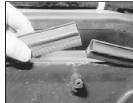
16.3 Remove the plenum chamber rubber seal
