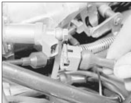
9.2 Disconnecting the cold start valve wiring multi-plug
