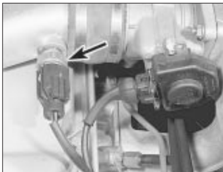
17.1 Charge air temperature sensor location (arrowed)
