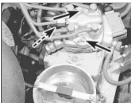
11.11 KE-Jetronic fuel distributor retaining screws (arrowed)
