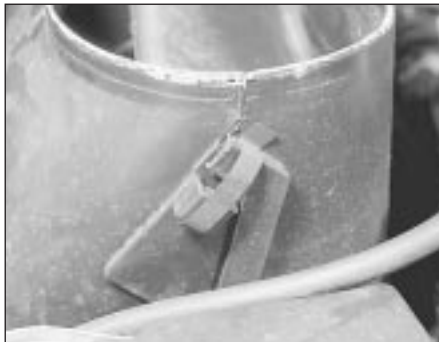
16.4a Release the retaining clips . . .
